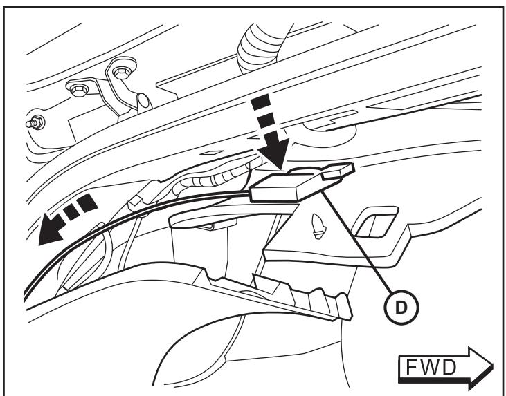
38. Secure the antenna module harness (D) along the existing vehicle harnesses inside the rear pillar with electrical tape.
