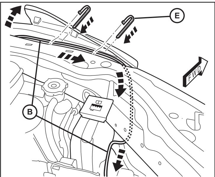
8. Route the switch harness (B) along the existing vehicle harnesses on the passenger side and back towards the rear of the engine compartment.
