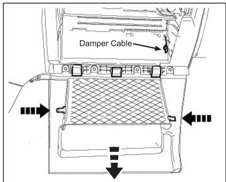
17. Use a trim stick to carefully unclip the inner storage shelf and remove it from the glovebox.
