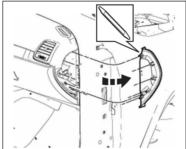
16. Open the glovebox door. Disconnect the glovebox damper cable. Press in on two (2) stop tabs. Rotate the door downward, release the door hinges and remove the glovebox door.
