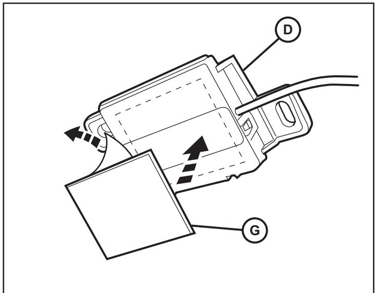
37. Peel off the remaining side of the double-sided adhesive panel (G) and mount the Antenna Module (D) to the inside of the headliner. Route the connector cable down towards the driver side pillar inside the trim panels.
