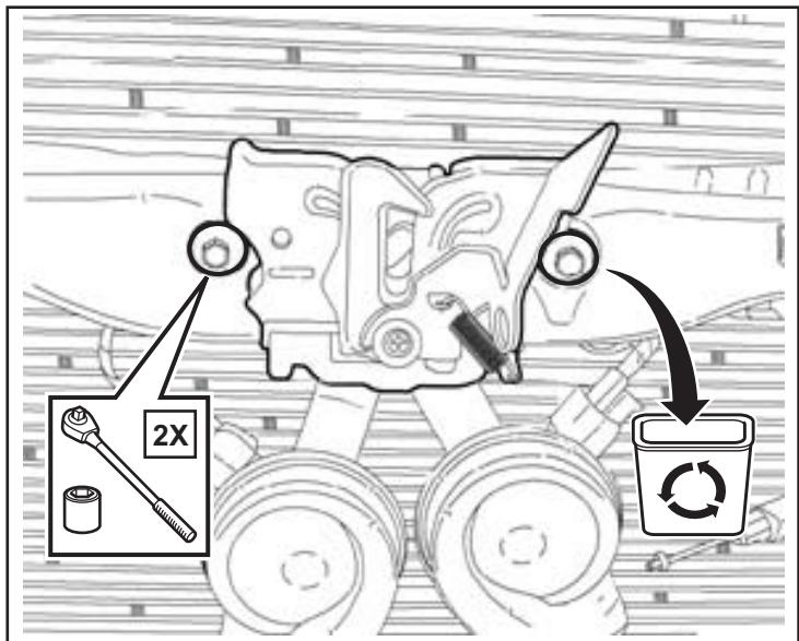
4. Carefully pry back the radiator cover panel. Disconnect and remove the hood latch release cable. Remove the hood latch assembly.
