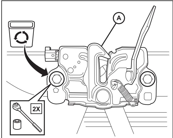
**NOTE:** A factory installed switch harness may be present. If so, detach the connector, route it under the crossmember and plug it in to the hood latch assembly, then proceed to Step 28.
