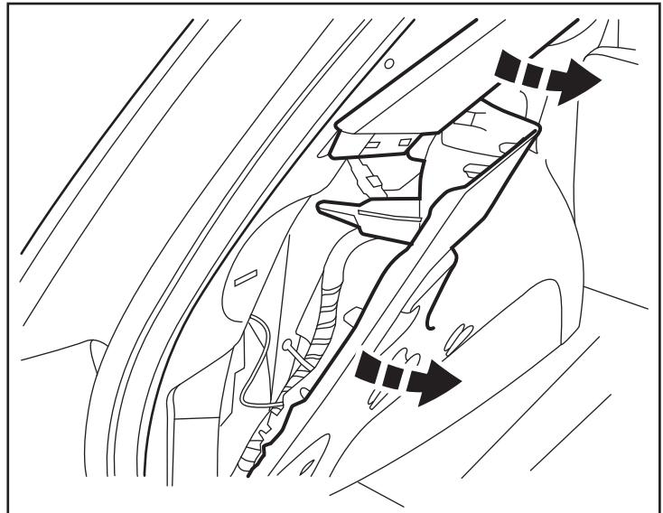
32. Locate the existing RF Hub Module on the driver side pillar of the rear hatch area. Disconnect all harness connectors. Remove two (2) hex nuts fasteners. Remove the RF Hub Module.
