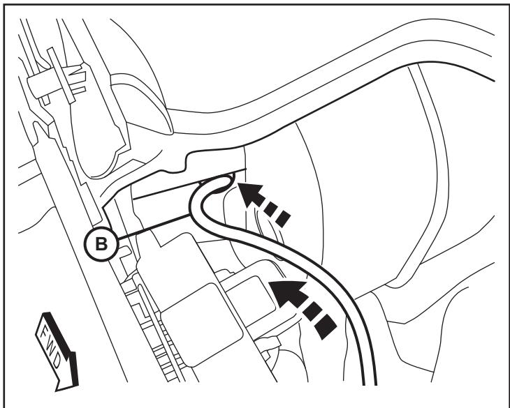
21. Cut an access hole through the grommet and feed the switch harness through the opening.
