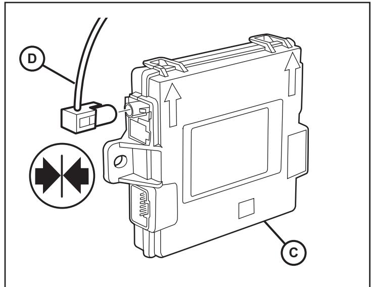
34. Place the new RF Hub Module (C) into position. Secure the RF Hub Module to the wall with two (2) hex nut fasteners (F) and reconnect all harness connectors.
