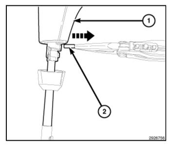
4. Using trim stick <u>C-4755</u> or equivalent, release the clip fasteners and separate the console bezel.
