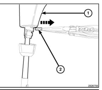
4. Align the ribs on knob (1) with slots in the chrome shroud (2) and seat the shroud fully. Angle on the shroud must match the angle on the knob before snapping in place.
