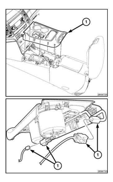
5. Disconnect the electrical connectors (1) and remove the shifter bezel.
