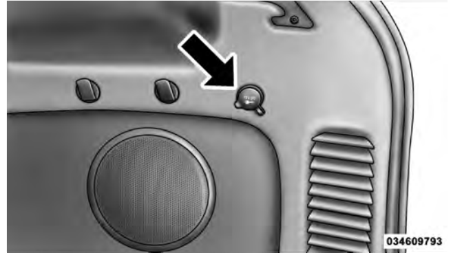
Rear Power Outlet
