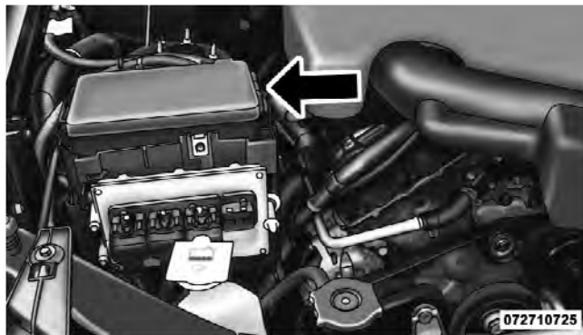
Totally Integrated Power Module
