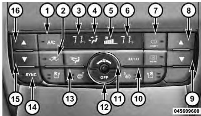
Automatic Temperature Control (ATC) Panel
