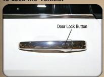
Both front door handles have LOCK buttons located on the outside of the handle. With one of the vehicle's Keyless Enter-N-Go Key Fobs located outside the vehicle and within 5 ft (1.5m) of the driver's or passenger front door handle, press the door handle LOCK button to lock all four doors and liftgate.
