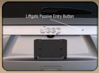
With a valid Keyless Enter-N-Go Key Fob within 3 ft (1.0m) of the liftgate, press the button located to the right of the liftgate handle to unlock the liftgate.
