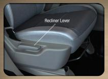
Lift the rear lever located on the outboard side of the seat, lean back and release when seat is in desired position.
