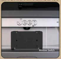
The liftgate flipper glass is unlocked when the liftgate is unlocked. To open the flipper glass, push up on the window switch located on the liftgate. When flipper glass is unlatched it will not completely raise, lift up on flipper glass handle to open.
