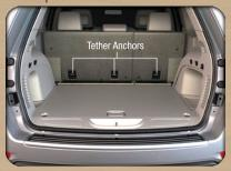
Tighten all three straps as you push the child restraint rearward and downward into the seat.
