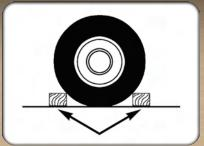
Block both the front and rear of the wheel diagonally opposite of the jacking position. For example, if changing the right front tire, block the left rear wheel.
