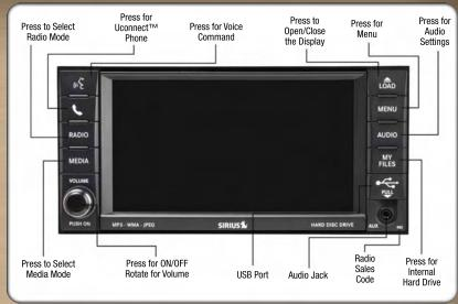
**NOTE:** Your radio may not be equipped with the Uconnect<sup>™</sup> Voice Command and Uconnect<sup>™</sup> Phone features. To determine if your radio has these features, press the Voice Command button on the radio. You will hear a voice prompt if you have the feature, or see a message on the radio stating "Uconnect Phone not available" if you do not.
