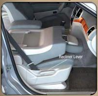
The front passenger seat can be folded flat to allow for extended cargo space.
