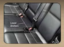
Loosen the child seat adjusters on the lower straps and tether straps so that you can attach the hook or connector to the lower tether anchorages more easily.
