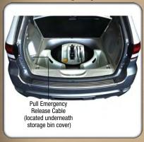
To manually open the fuel door, remove the storage bin and pull the release cable located in the rear cargo area.
