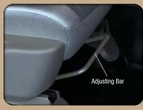
Lift up on the adjusting bar located at the front of the seat near the floor and release when seat is in desired position.
