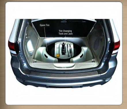
The scissor-type jack and tire changing tools are located in the rear cargo area, below the load floor.
