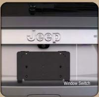
The liftgate flipper glass is unlocked when the liftgate is unlocked. To open the flipper glass, push up on the window switch located on the liftgate. When flipper glass is unlatched it will not completely raise, lift up on flipper glass handle to open.
