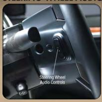
The steering wheel audio controls are located on the rear surface of the steering wheel.
