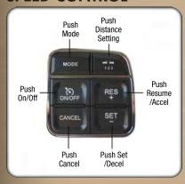
The speed control switches are located on the steering wheel.
