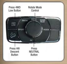
The Quadra-Trac II®/Quadra-Drive II® transfer case is fully automatic in the normal driving 4WD HI mode. The Quadra-Trac II®/Quadra-Drive II® transfer case provides three mode positions:
