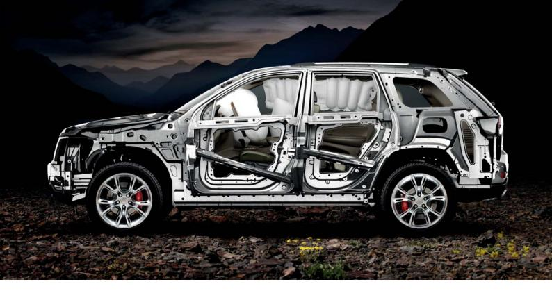
A SAFE, SECURE AIR BAG SYSTEM. ALWAYS STANDARD: FULL-LENGTH SIDE-CURTAIN, SEAT-MOUNTED SIDE THORAX, AND ADVANCED MULTISTAGE FRONT AIR BAGS ALL WORK IN TANDEM TO HELP PROVIDE PROTECTION.
