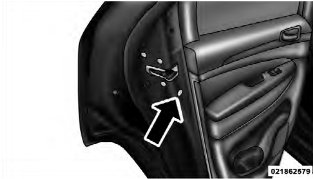
Child-Protection Door Lock Location
