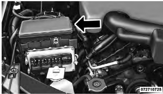
Totally Integrated Power Module
