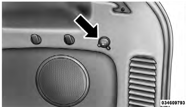
Rear Power Outlet
