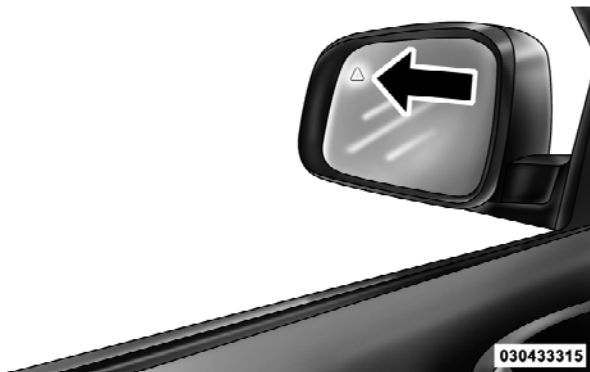
Warning Light Location
