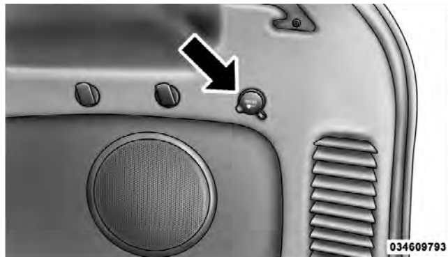
Rear Power Outlet
