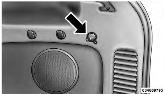
Rear Power Outlet
