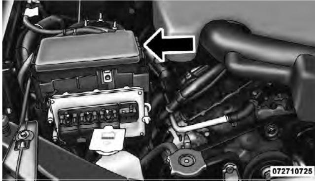
Totally Integrated Power Module
