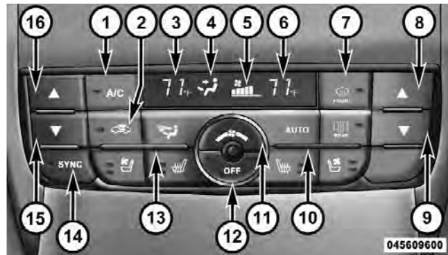
Automatic Temperature Control (ATC) Panel
