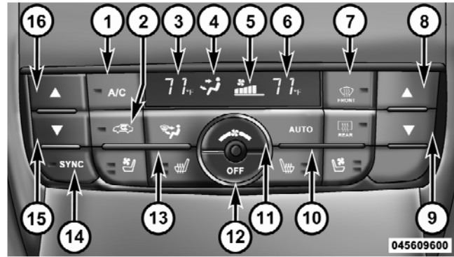
Automatic Temperature Control (ATC) Panel
