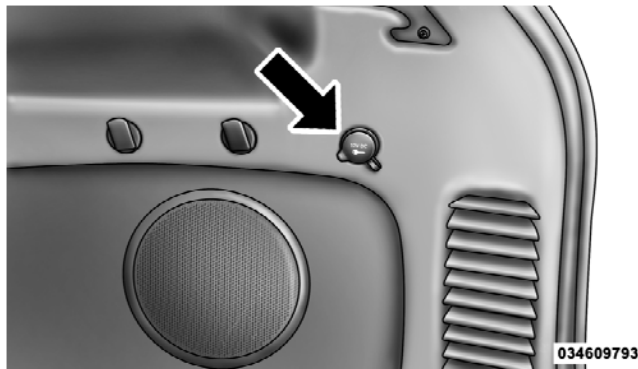
Rear Power Outlet
