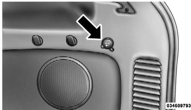
Rear Power Outlet
