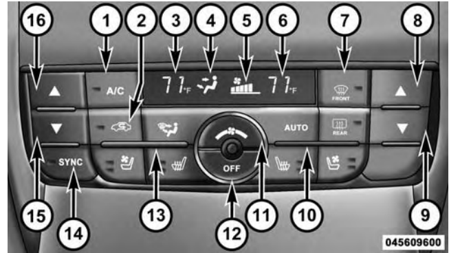
Automatic Temperature Control (ATC) Panel
