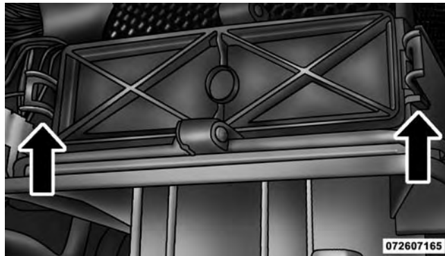
A/C Air Filter Replacement
