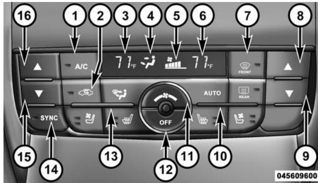
Automatic Temperature Control (ATC) Panel
