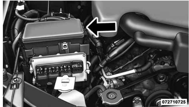
Totally Integrated Power Module
