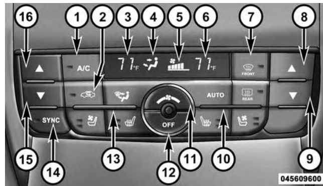
Automatic Temperature Control (ATC) Panel
