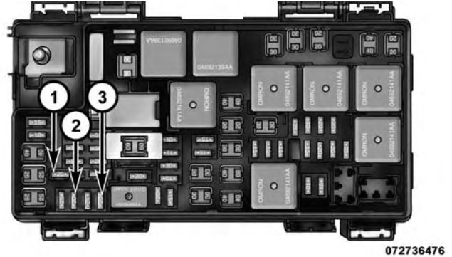
Power Outlet Fuse Locations
