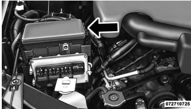
Totally Integrated Power Module
