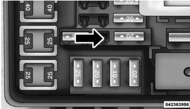
Power Outlet Right Rear Quarter Panel Fuse
