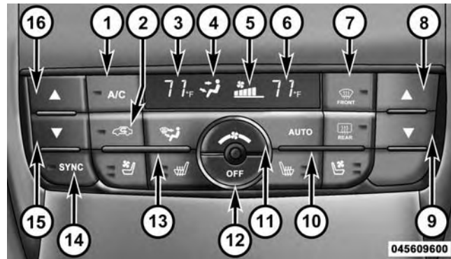
Automatic Temperature Control (ATC) Panel
