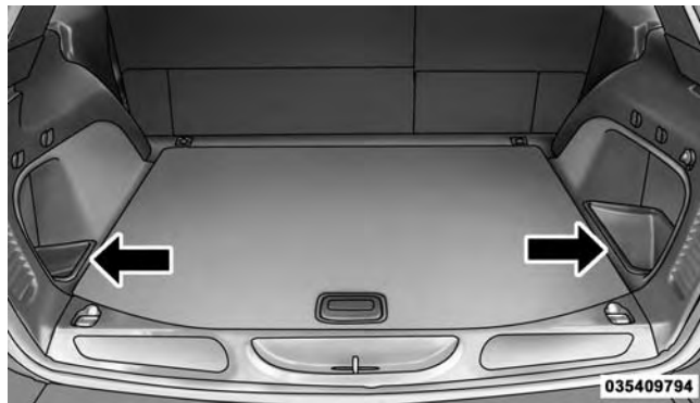
Rear Storage Bins
