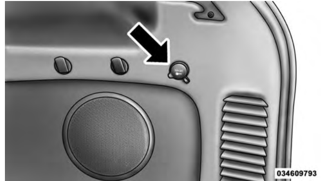
Rear Power Outlet
