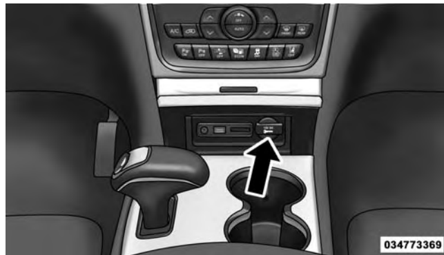
Front Power Outlet
