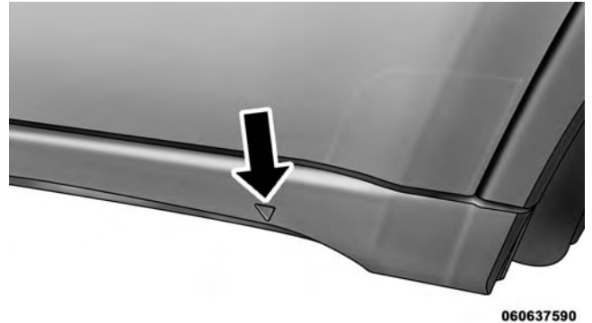
Lift Point Symbol On Sill Molding
