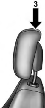
3 — Final Downward Movement To Engage Locking Mechanism
