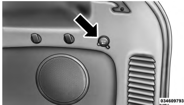
Rear Power Outlet
