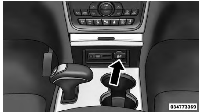
Front Power Outlet
