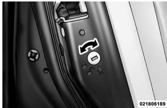
Child-Protection Door Lock Function
