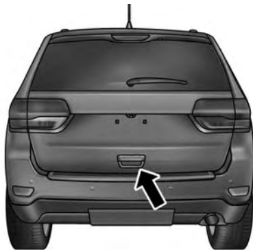
Electronic Liftgate Handle/Liftgate Passive Entry Location
