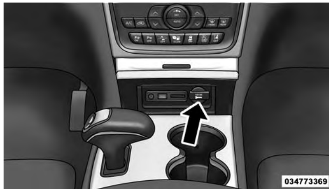
Front Power Outlet
