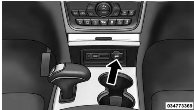
Front Power Outlet
