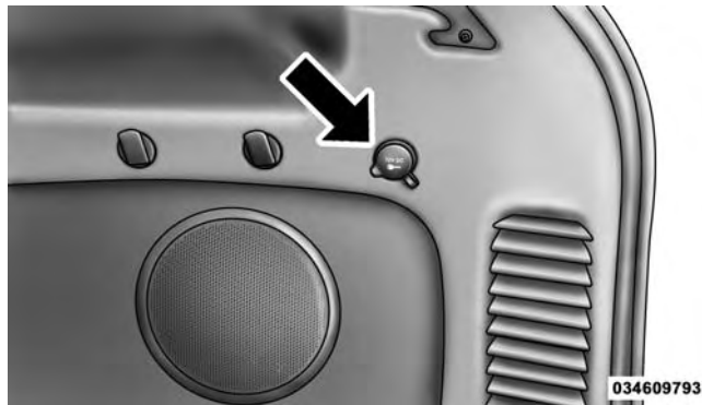
Rear Power Outlet
