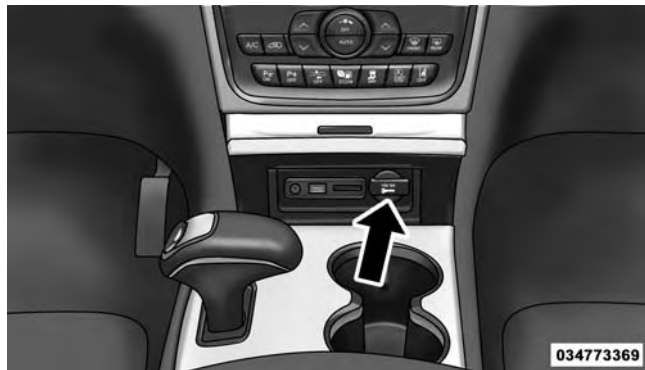
Front Power Outlet
