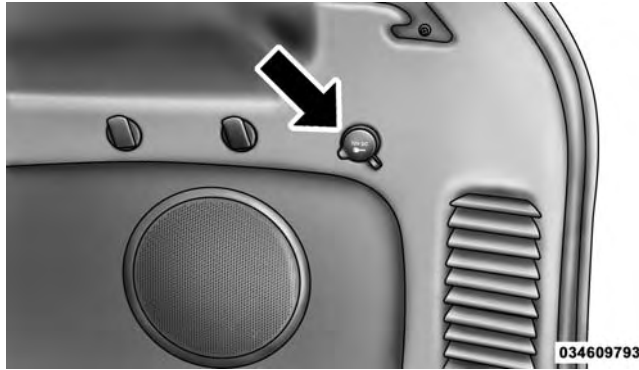
Rear Power Outlet
