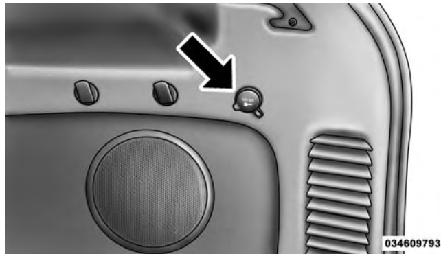
Rear Power Outlet
