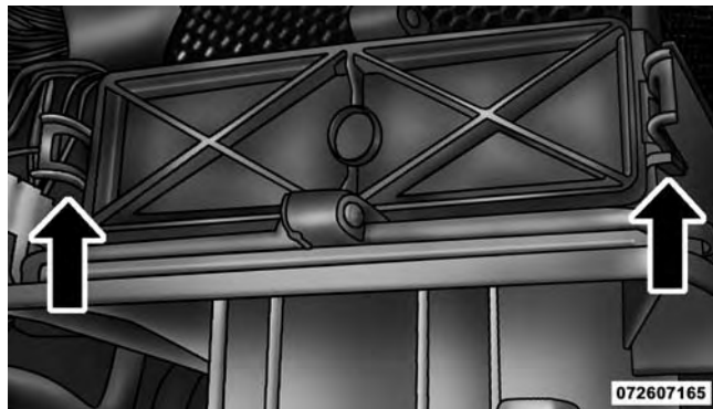
A/C Air Filter Replacement
