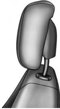
Active Head Restraint (Normal Position)
