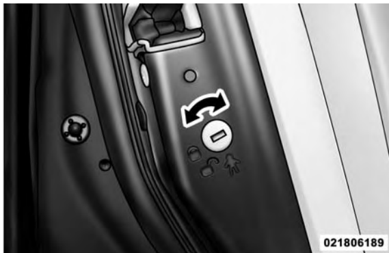
Child-Protection Door Lock Function
