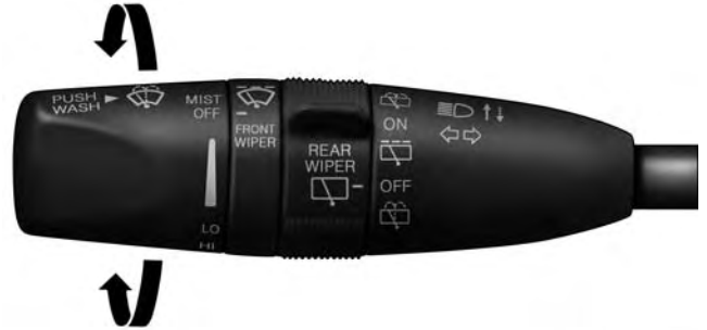
Windshield Wiper Operation
