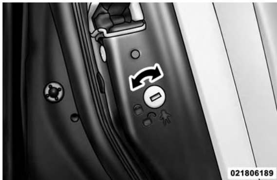
Child-Protection Door Lock Function
