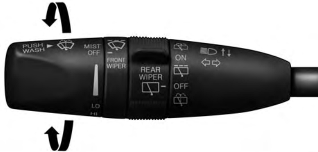
Windshield Wiper Operation
