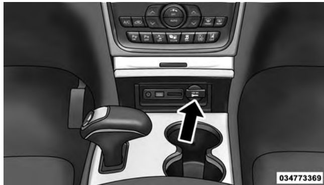
Front Power Outlet
