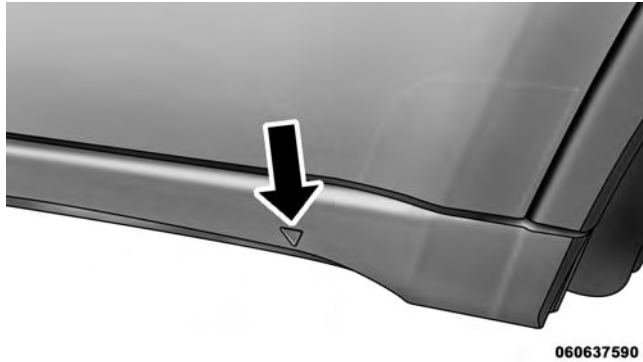
Lift Point Symbol On Sill Molding
