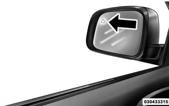
Warning Light Location
