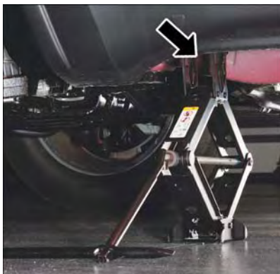
Front Jacking Location
