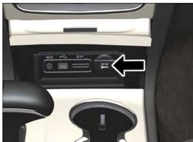
Front Power Outlet
