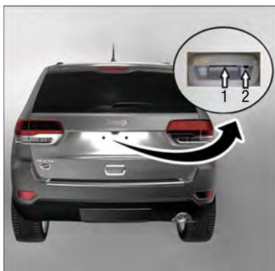
Electronic Release Switch Location
