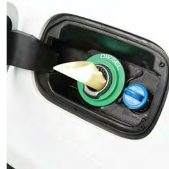
Emergency Fuel Fill Location
