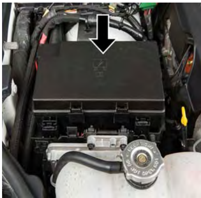
Power Distribution Center Power Distribution Center
