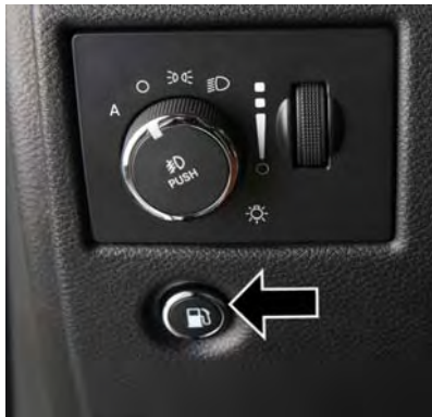
Fuel Filler Door Release
