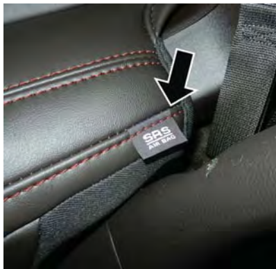
Front Supplemental Seat-Mounted Side Air Bag Label
