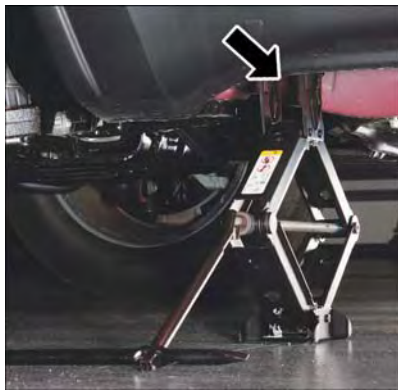
Front Jacking Location
