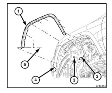
4. Remove the 1/4 turn fasteners (1) and separate the lower wheel liner from the fascia.
