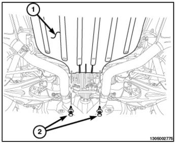
3. Remove the plastic rivets (1) that secure the wheel liners to the rear fascia.
