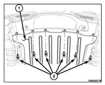
2. Remove the front push pin fasteners (2) and remove the rear belly pan (1).
