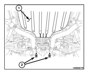
11. Install the rear push pin fasteners (2) securing the rear belly pan (1) to the fascia.
