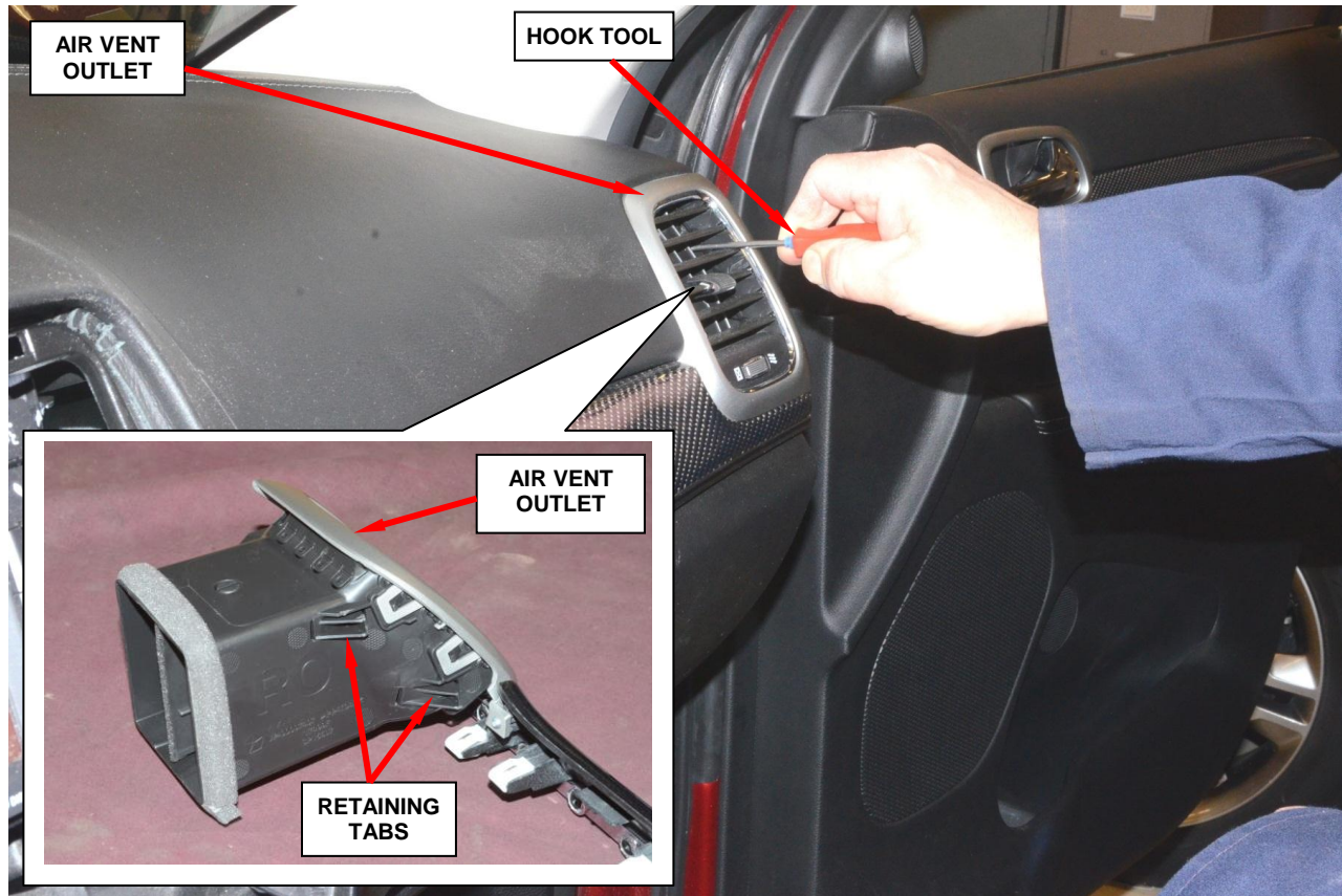
Figure 3 – Disengage the Air Vent Outlet Retaining Tabs (two per side)
