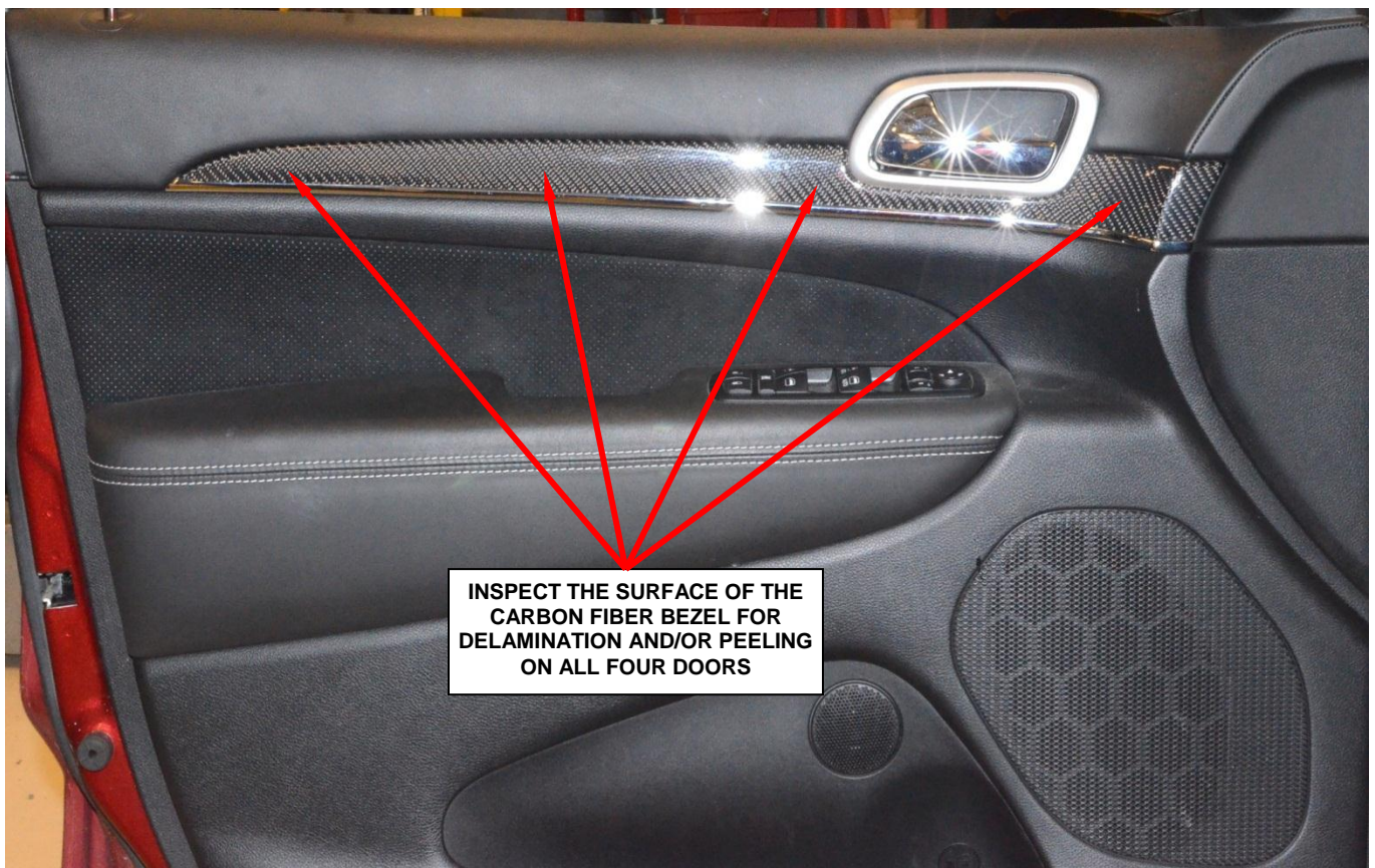
Figure 13 – Inspect All Door Trim Panel Carbon Fiber Bezels (left front door shown)
