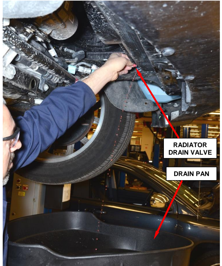
Figure 2 – Drain Coolant into Drain Pan
