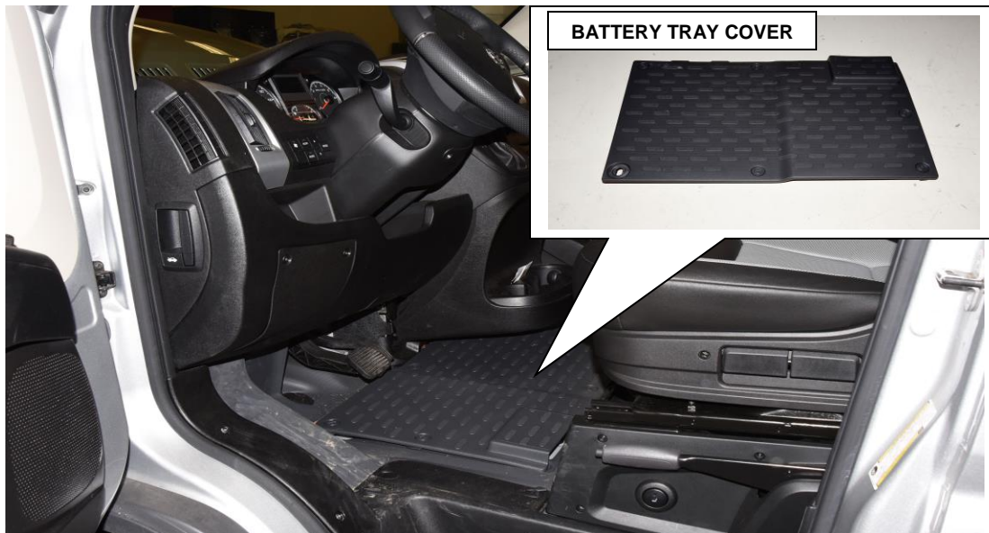
Figure 24 – Battery Tray Access Cover
