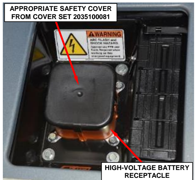
Figure 17 – High-Voltage Battery Receptacle Safety Cover
