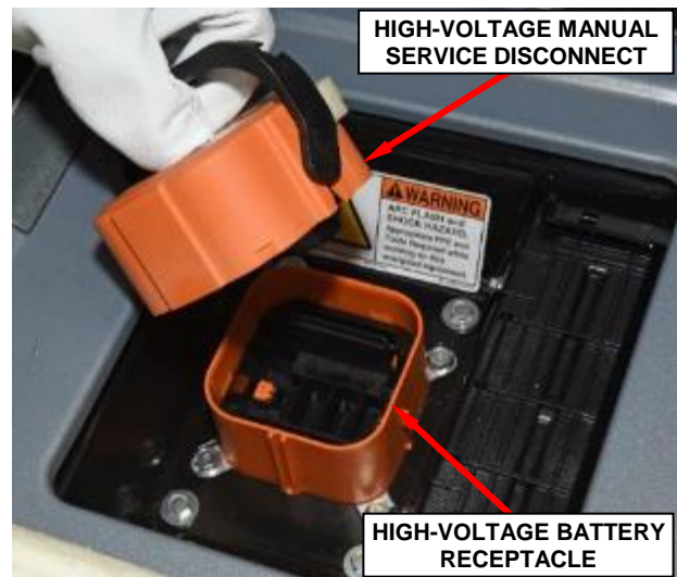
Figure 16 – High-Voltage Manual Service Disconnect and Receptacle
