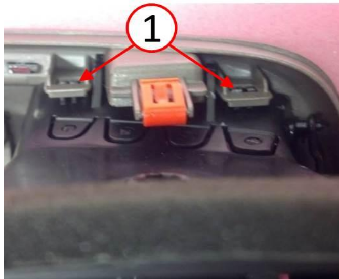
Fig. 3 HVAC Outlet Upper Attachment
