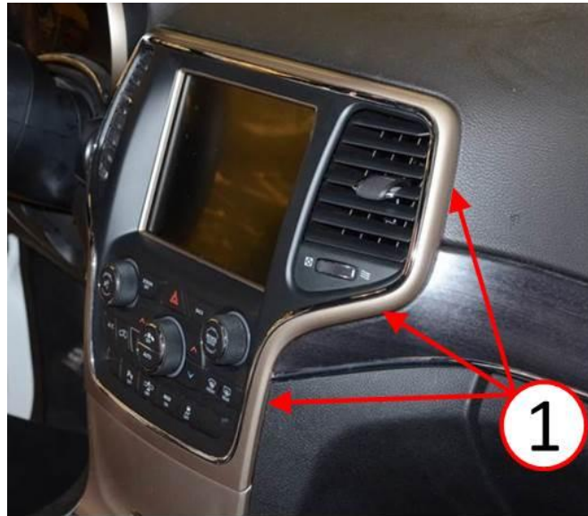
Fig. 15 ICS Bezel Installation Inspection
