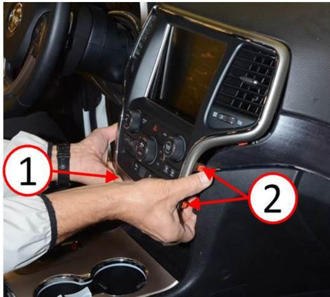
Fig. 10 ICS Bezel Removal Lower
