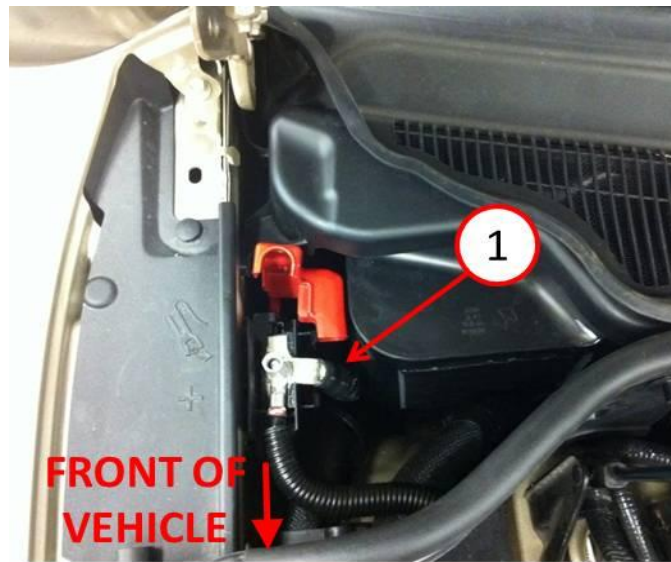
Fig. 2 Battery Positive Jumper Post
