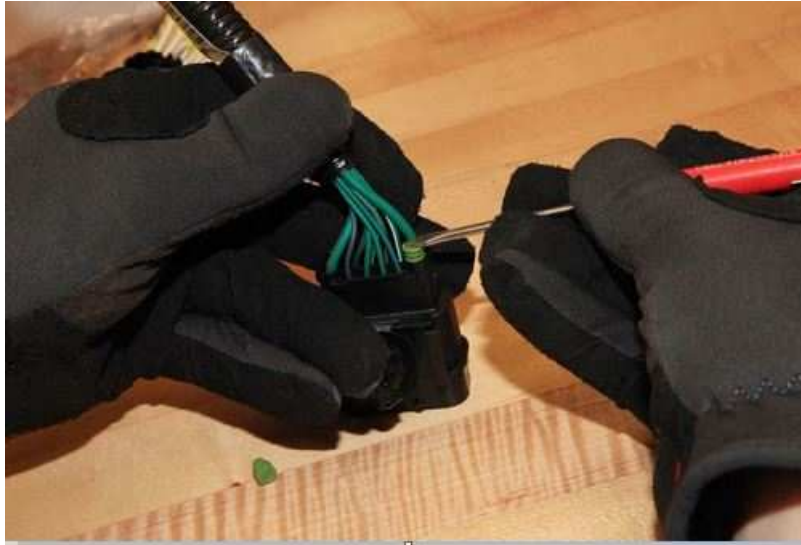
Fig. 2 Installing Dummy Cavity Plug
