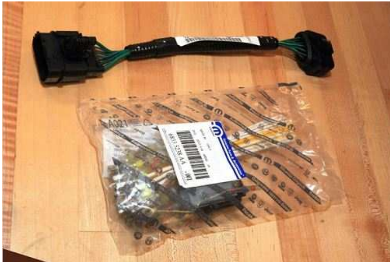
Fig. 3 Connector Terminal Repair Kit and ELSD Jumper Harness
