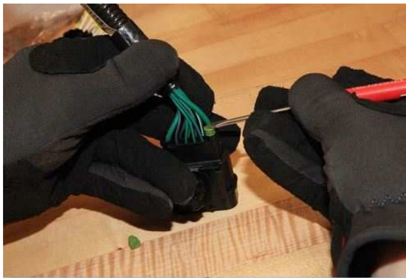
Fig. 4 Installing Dummy Cavity Plug
