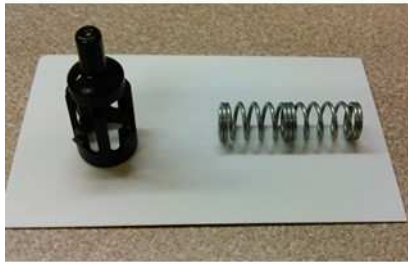
Fig. 2 New Oil Pressure Relief Valve
