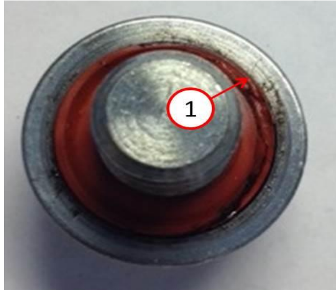
Fig. 2 Damaged Rubber Seal
