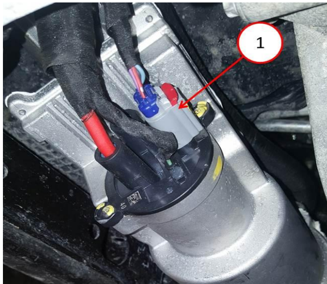
Fig. 2 WD and WK EPS Module Connector
