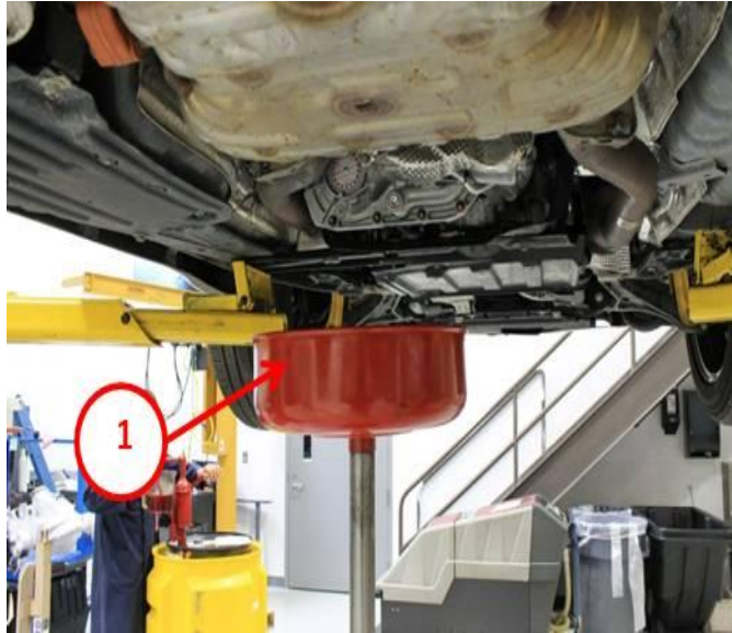
Fig. 1 Drain Transfer Case Fluid
