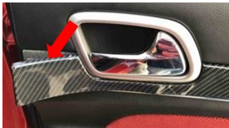
Fig. 1 Applique Delaminating Example
