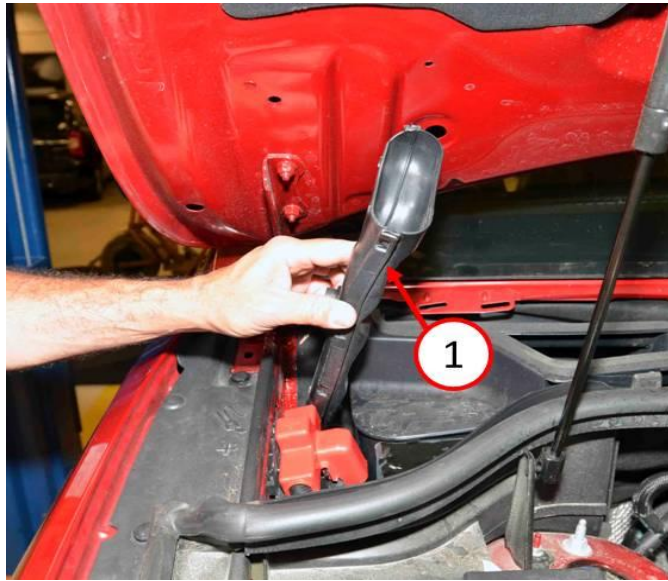
Fig. 7 Cowl Drain Trough Removal
