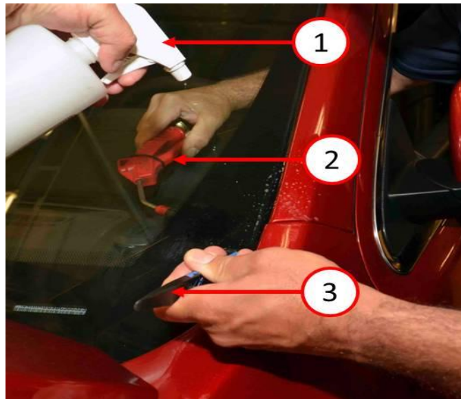
Fig. 3 Leak Check Lower Windshield Seal
