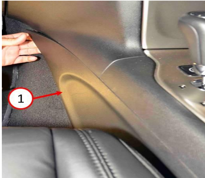
Fig. 5 Console Side Cover Removal
