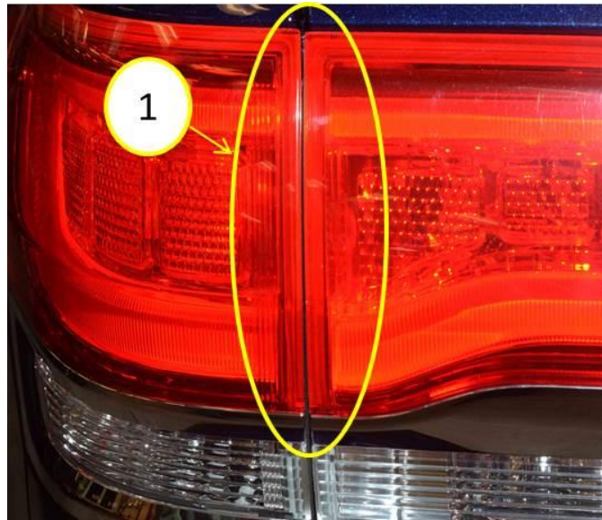
Fig. 1 Too Close Of Gap Clearance
