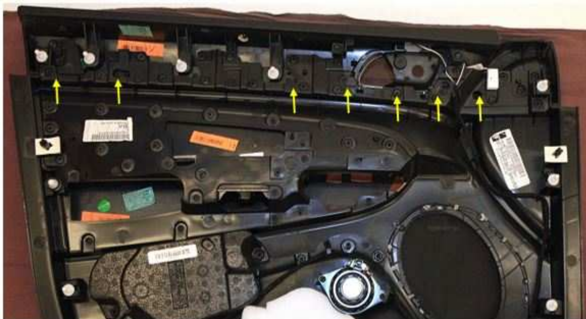
Fig. 10 Location of Seven Retaining Screws on the Front Door Panel
