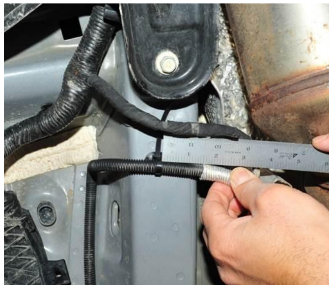
Fig. 4 MEASURE FROM THE FOIL FOR TIE LOCATION
