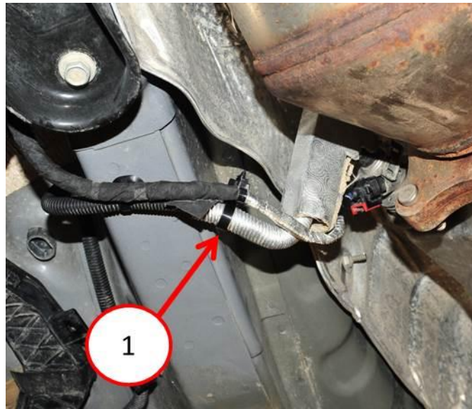
Fig. 6 WIRE TIES INSTALLED
