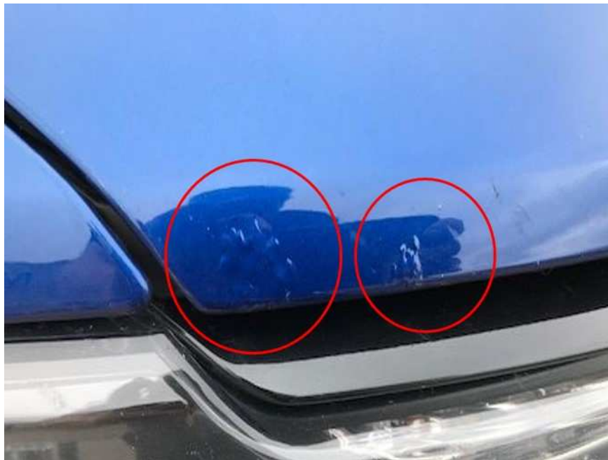
Fig. 1 Examples of Corrosion Along Leading Edges
